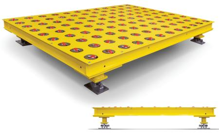
Rice Lake's RoughDeck CC castor cargo scale has 360-degree castors that swivel, making it easy for the operator to move and position cargo from any direction on and off the scale. The CC castor cargo scale has four removable top panels for accessing load cells
