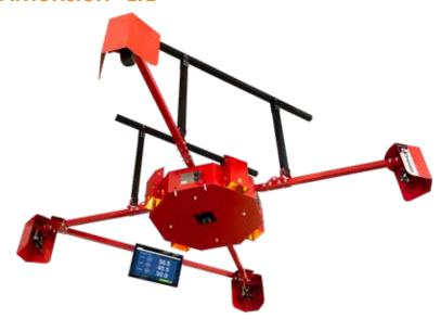
The iDimension LTL uses advanced sensing technology to determine the cubic dimensions of freight, ensuring that freight code compliance is recorded and declared. Ideal for LTL carriers and companies with a high percentage of product shipped via pallet or crate, the iDimension LTL removes the potential for human error when taking measurements. The extra labor of manually determining dimensions is eliminated, as the iDimension LTL accurately captures freight dimensions in less than two seconds.
